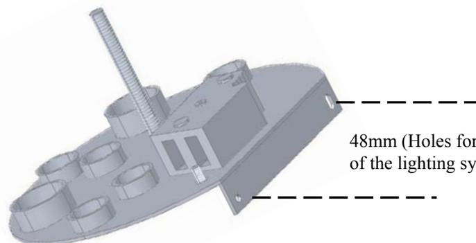
48mm (Holes for wall implantation of the lighting system apparatus).
